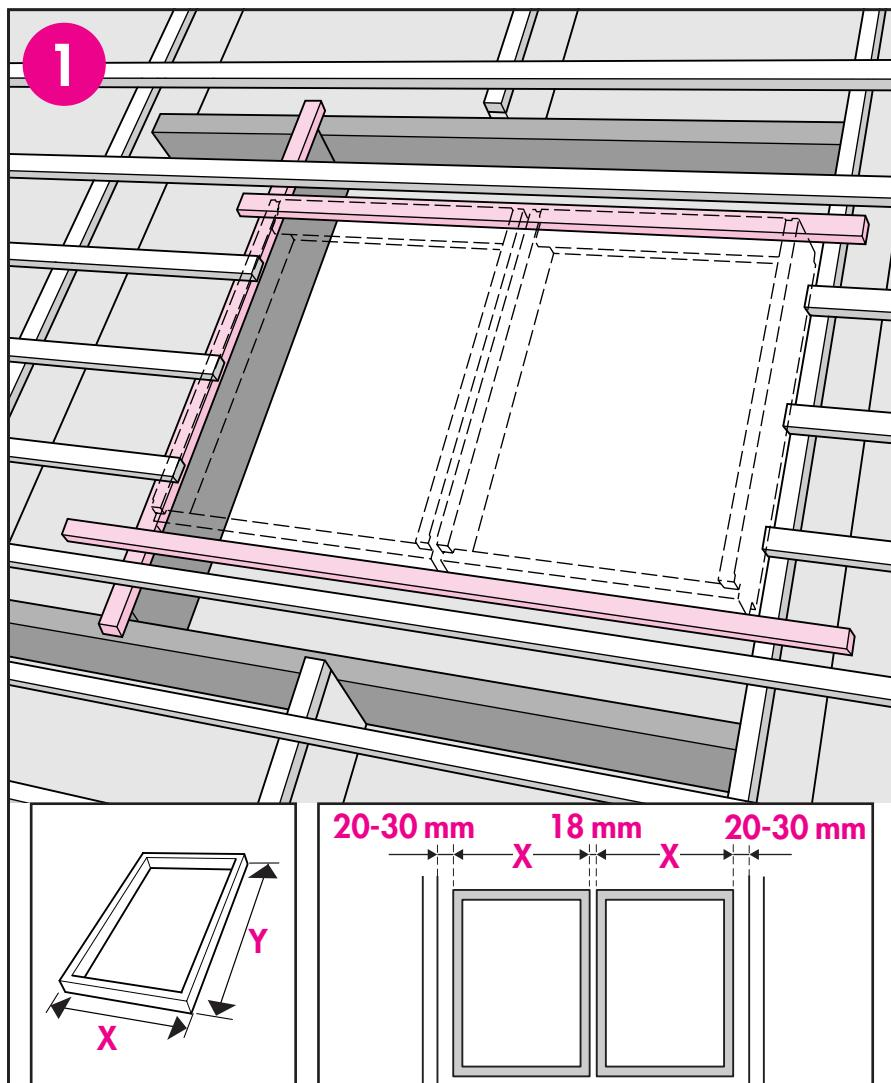
**ENGLISH:** Position of windows to be in relation to the relevant roofing material: See instructions enclosed with the windows. Position of trimmers and support battens: See information below.
