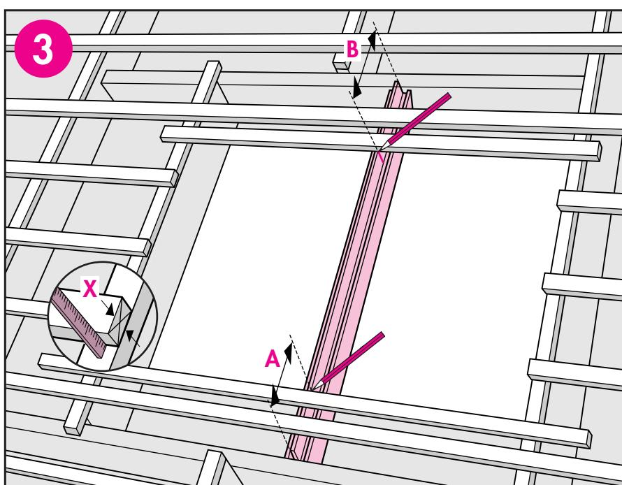
**ENGLISH:** Adjust EBY at the ends. The measurement **X** must be maximum **40 mm** when cutting out the EBY.
