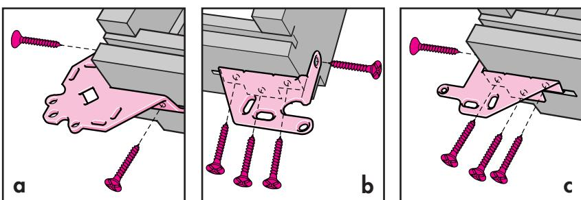
**ENGLISH:** Fit seals supplied into the two window rebates to be positioned onto the EBY (1). Fix brackets supplied with the windows to the frame sides opposite the EBY (a). Fix brackets supplied with the flashing to the frame sides facing the EBY (b, c).
