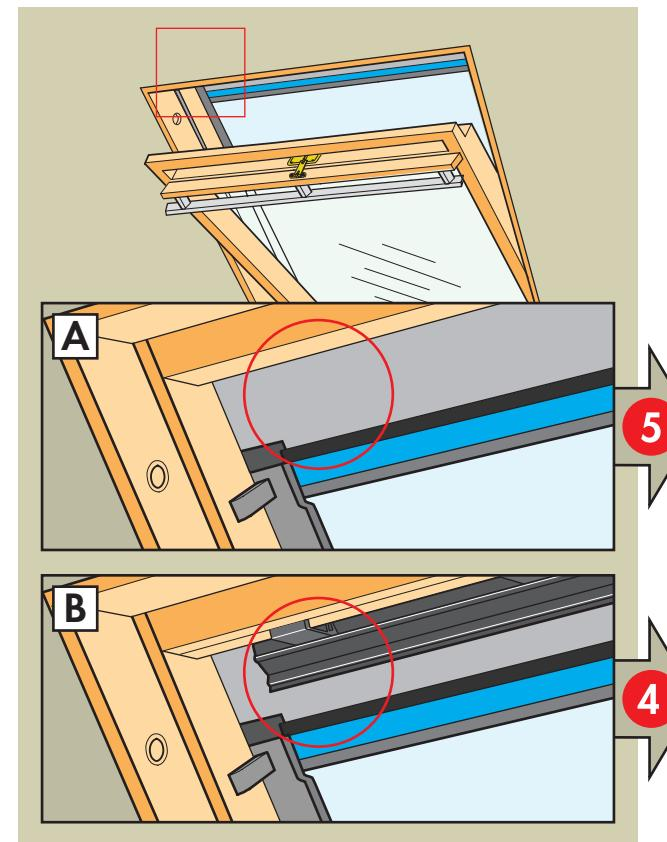
**English:** **A:** Window does **not** have a screen profile: Continue with step **5**. **B:** Window **has** a screen profile: Continue with step **4**.
