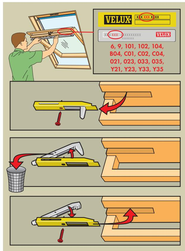
**English:** Find the window size on the data plate. For the above-mentioned window sizes **only**, replace the barrel bolt with barrel bolt supplied.
