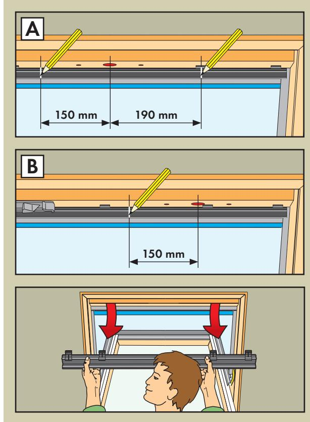
**English:** A: Window with **one** striking plate: Mark screen profile as shown. B: Window with **two** striking plates: Mark screen profile as shown.
