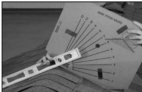
1. To determine roof pitch, place gauge on peak of roof as shown. Position straight edge as shown. Read roof pitch from printed gauge parallel to bottom of straight edge.
