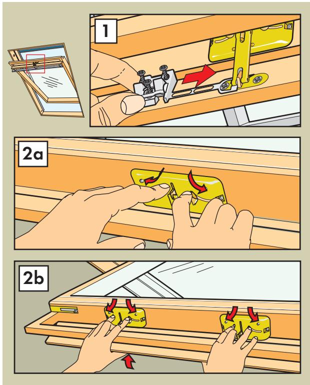
**English:** Fit the bracket onto the headlock (windows with two headlocks: onto the right headlock) (1). Disengage the lock: Windows with one headlock (2a), windows with two headlocks (2b).
