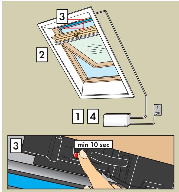
**English:** Connect control system to mains supply (1). Open window manually (2). Press the test button on window operator for at least 10 seconds. The window operator chain runs briefly back and forth (3). Disconnect mains supply (4).
