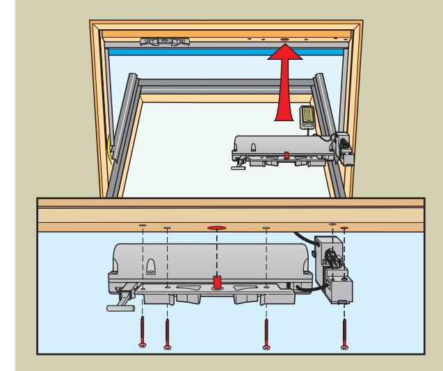
**English:** Fit the window operator where the striking plate was fitted using the four screws supplied. Fit the rain sensor according to instructions for rain sensor or directions for use.
