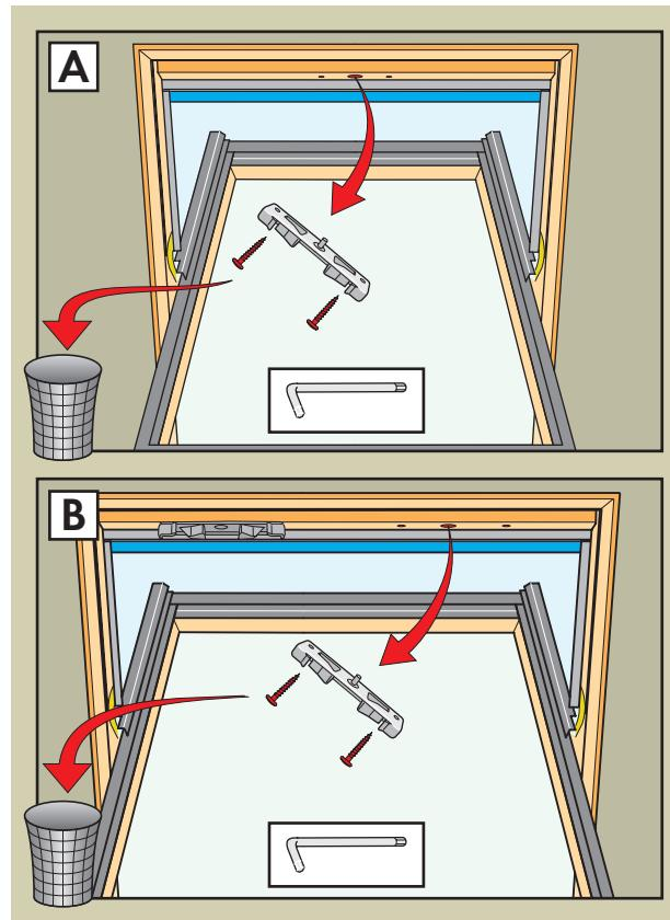
**English:** **A:** Window with **one** striking plate: Remove striking plate and discard along with screws. **B:** Window with **two** striking plates: Remove only the right hand striking plate. Use TORX key supplied if necessary.
