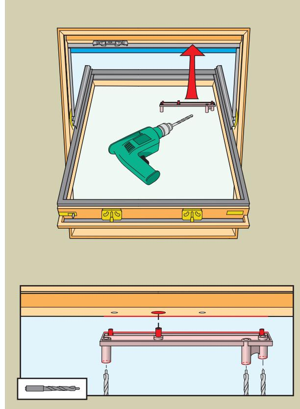
**English:** Position drilling jig where the striking plate was fitted. Drill pilot holes using drill bit supplied.
