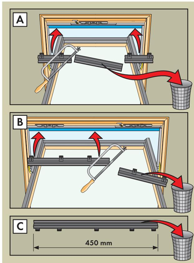
**English:** A: Window with **one** striking plate: Adjust screen profile as shown and refit. Close the window. B: Window with **two** striking plates: Adjust screen profile as shown and refit. Close the window. C: Discard screen profile if it measures 450 mm or less.
