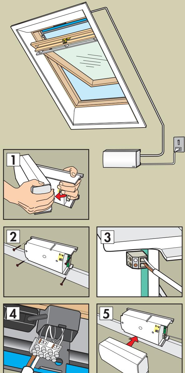
**English:** Remove cover from control unit (1). Fix control unit to wall (2). Connect cable to control unit (3) and run cable from control unit to terminal block where you can choose to connect it to A (brown/white) or B (brown/white) (4). Only **one** 2-core cable should be used. The terminal distributes the electricity to other products which may be fitted on the window and are also connected to A or B. Replace control unit cover (5).
