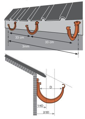
Place the necessary support brackets with a distance of + 33cm.
