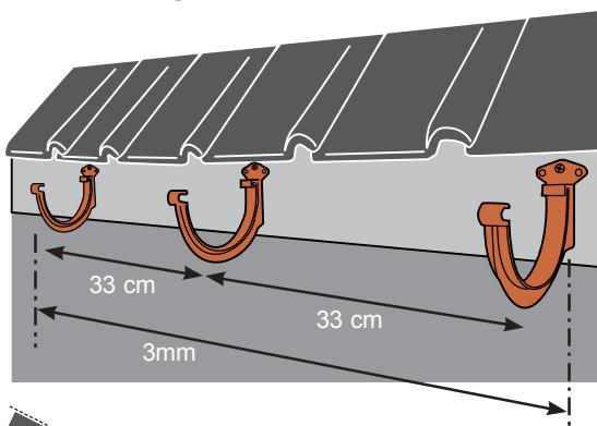
Place the necessary support brackets with a distance of  $\pm 33\text{cm}$ . It's recommended to attach 3 support brackets per meter, because they carry the full gutter system. If the roof often has to carry much weight (eg snow), it's recommended to place the support brackets at a shorter distance . Attach the support brackets, while descending 3 mm in the direction of the drainpipes.
