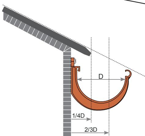
The length of the cornice should be at least 1/4 and no more than 2 / 3 of the width of the gutter (D).
