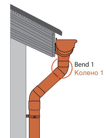
In case of a sloping roof, connect the outlets and pipes with two bends and use a custom measured pipe between the bends. **Attention!** For future replacements or repairs it's recommended not to glue bend 1 during installation.
