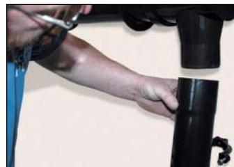
Attach the pipe to the outlet.
