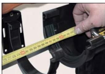
Measure the length of the gutter to the "limit position".
