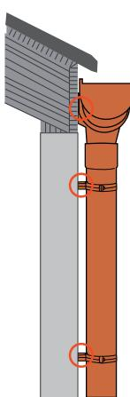
The wall-connections of the outlets and fixos are on one line. This simplifies and speeds the installation of straight drain pipes.
